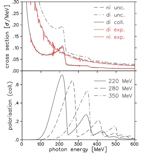
Fig 2: Nickel and diamond cross sections and polarization prediction for 3 crystal settings
